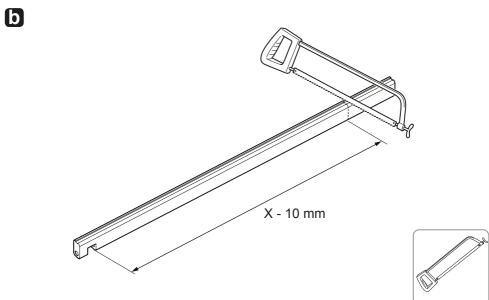
(a) Cut the bracing bar to the measured dimension 'X' minus 10 mm (X - 10 mm).e.g. If the measured dimension is 760 mm then cut the bracing bar to 750 mm
