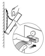
**15.** Connect ribbon cable to the inside of the cover.
