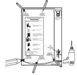
Use template provided to mark and drill required fixing holes. Screws and plugs are supplied for 4 holes.
