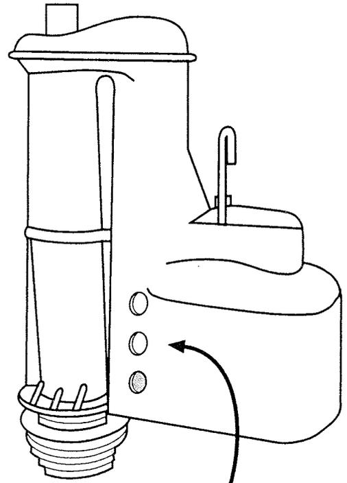
Press flush volume selector firmly into position to close the required holes.
