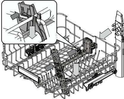
The Top Rack has a fixed wash tube with all the wash nozzles facing upward. To clean it you can slide the rack out and with a tweezer remove items that may be lodged in the nozzles.
