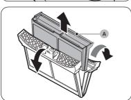
Open the outer filter and remove the inner filter (A).
