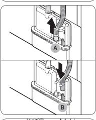
**1.** Remove the drain hose from **hole** (A), and insert it into **part** (B).
