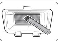
**4.** Clean the heat exchanger with the provided cleaning brush or a vacuum cleaner with a brush attachment. Take care not to bend or damage the heat exchanger fins when cleaning. This may lead to a decrease in drying performance.
