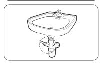
**2.** Connect the hose adapter directly to the drain pipe of the wash basin.
