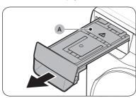
1. Using both hands, pull the water tank (A) forward to remove.
