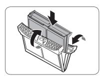
**5.** Put the inner filter into the outer filter, and then reinsert the lint filter into the original position.
