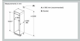
measurements in mm Recommended gap dimensions for flat hinges
