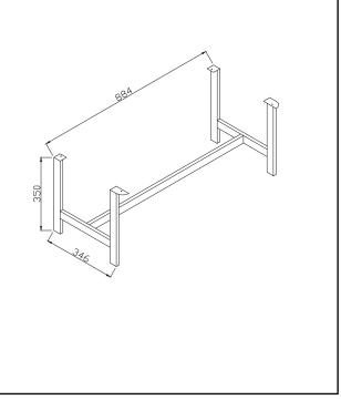
Dimensions (Measurements in mm)
