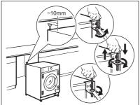
**2.** Adjust the anti-tilting device so that the distance from the counter is 10mm. Loosen the nut counterclockwise with a 3mm wrench. Adjust the height and turn the nut clockwise to fix it.
