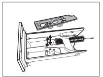
3. Make sure that all detergent residue is removed from the upper and lower part of the recess. Use a small brush to clean the recess.
