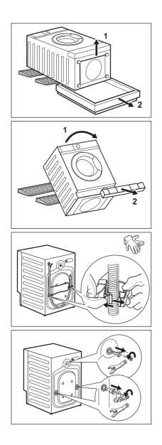
**3.** Remove the polystyrene protection from the bottom.
