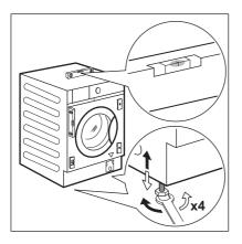
1. Install the appliance on a flat hard floor.
