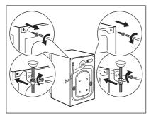
**1.** Remove the screws of the top cover on the rear of the appliance and install the anti-tilting device as shown in the drawing.
