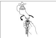
**3.** Connect the hose to the back of the appliance. Do not turn the inlet hose downwards, but turn it left or right depending on the position of your water tap.
