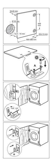
Set the position of the lower hole respecting dimensions and distances shown in the drawing (449 mm).
