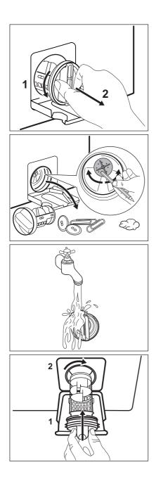
6. Turn the filter anti-clockwise to remove it
