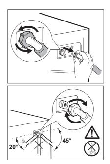
When you drain the water with the emergency drain procedure, you must activate the drain system again:
