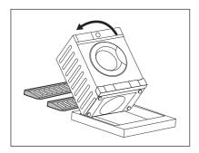
**1.** Put two polystyrene packaging elements on the floor under the appliance.
