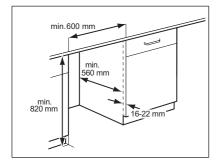
This appliance has been designed to be built into the kitchen furniture. See the minimum recess dimensions in the drawings.
