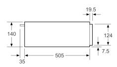
Compact ovens with an appliance height of 455 mm can be installed above a warming drawer. An intermediate floor is not required.
