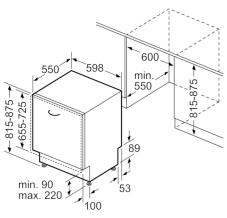
measurements in mm
