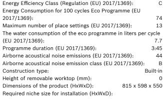
815-875 x 600 x 550 Depth with open door 90 degree (mm): 1150 Yes - all from front Adjustable feet: Maximum adjustability feet (mm): Adjustable plinth: both horizontal and vertical Net weight (kg): 42.830 Gross weight (kg): 45.0 Connection rating (W): 2400 Current (A): 10 Voltage (V): 220-240 Frequency (Hz): 50; 60 Length of electrical supply cord (cm): 175 GB plug Plug type: Length inlet hose (cm): 165 Length outlet hose (cm): 190 EAN code: 4242005270309 Full-integrated Installation type:
