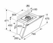
Socket can be fitted to the side of or above the appliance
