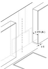
A: Max. depth of side upper cabinets (incl. door) due to installation of glass plate
