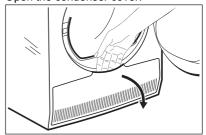
Turn the levers to unlock the condenser lid.
