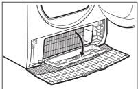
If necessary, remove the fluff from the condenser and its compartment. You can use a vacuum cleaner with a brush attachment.
