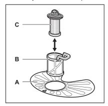
Turn the filter (B) counterclockwise and remove it.
