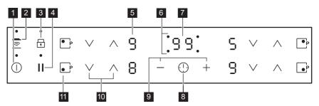
Use the sensor fields to operate the appliance. The displays, indicators and sounds tell which functions operate.
