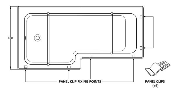
3. WHEN FITTING THE END PANEL, TAKE A MEASUREMENT FROM THE BACK EDGE OF THE FRONT PANEL TO THE WALL (DIM 'A')
