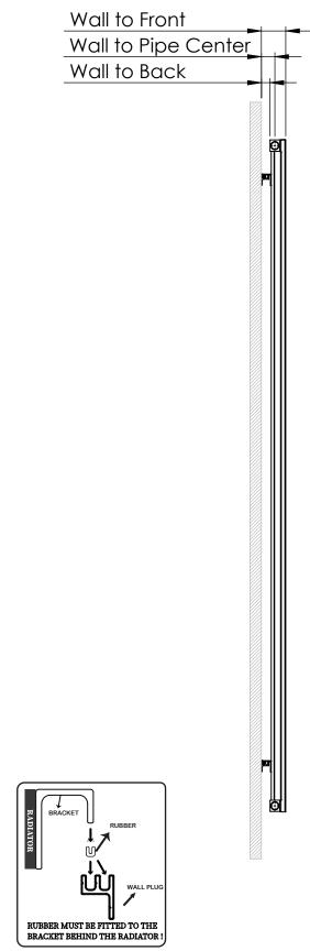
Since the wall mountingset has two stages, the distances from the wall are indicated in the table below according to the two stages
