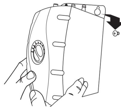
Hang new tank on mounting bracket or screws.
