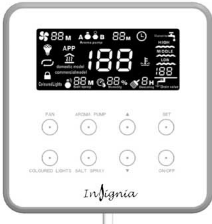
Figure 4 AIO control panel
