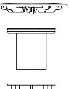
This waste provides a flow rate greater than 32L per minute when tested in accordance with EN274-2:2002. The flow rate can be seriously impaired if an adequate fall is not maintained throughout the length of the waste pipe.
