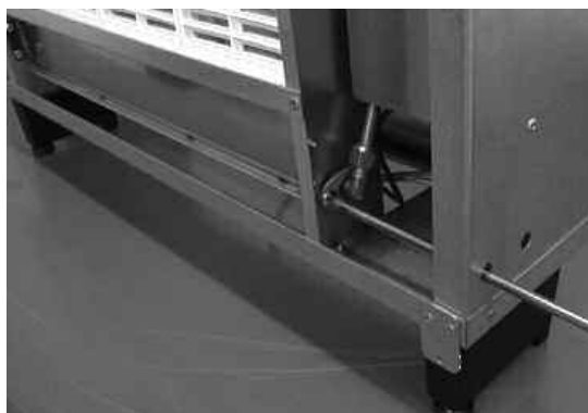
Fig. 11 Injector fixing bracket removal
