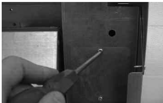
Fig. 13 Service Plate Removal
