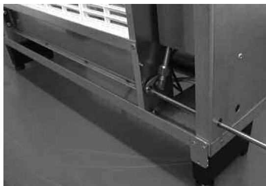
Fig. 11 Injector fixing bracket removal
