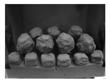
f) Select the remaining four small coals and arrange along the rear of the fuelbed, directly behind the third row of coals. See fig. 6 below.
