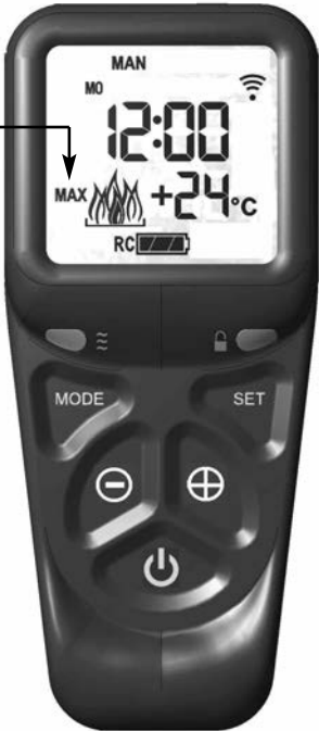
Fig. 3 - “MAX” & large flame symbol displayed
