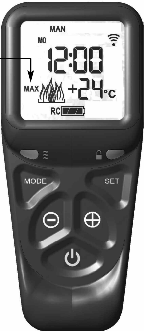
Fig. 35 - “MAX” & large flame symbol displayed
