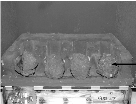
Front Row Coal Positioning - Side Profile
