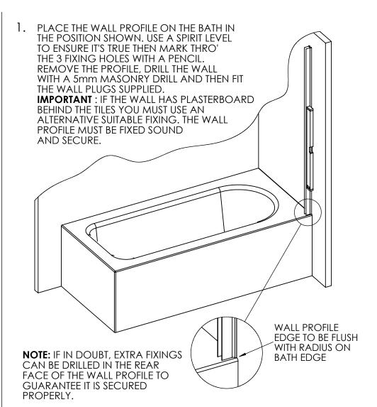
2. NOW SLIDE THE SCREEN ASSEMBLY INTO THE WALL PROFILE. THE BOTTOM EDGE OF THE GLASS PANEL **MUST** BE PARALLEL TO THE BATH TOP FACE. YOU CAN MAKE A WOODEN SPACER (18mm) TO FIT UNDER THE GLASS SO THERE IS AN EQUAL GAP ALL THE WAY LONG. THE SPACER WILL SUPPORT THE SCREEN PARALLEL WHILST YOU FIX IT IN PLACE AND THEN REMOVED.
