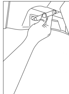
3, using a pen to mark the basin wall huge holes positions on wall, and pedestal install position line on floor.
