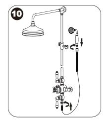
10.Connect the hand shower and hose to the mixer depending on the design, check that all connections are tight.
