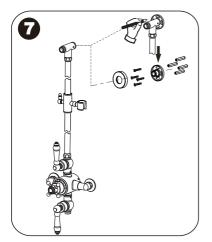
7.Fix the wall bracket onto the elbow, then put against the wall and mark the position of the wall bracket. Use this as a guide to mark 4 x fixing holes.
