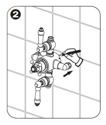
2.Put the shower mixer against the wall and mark the position of the valve body. Then using a hexagon spanner unlock the securing grub screws to remove the mounting bracket from the shower mixer.
