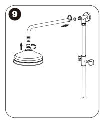
9.Insert the shower arm into the elbow and lock the nut, fit the shower head onto the shower arm.
