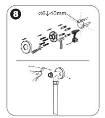
8.Drill 4 x holes in the wall then insert the plastic wall plugs and attach the wall bracket, using the supplied screws. Ensure the wall bracket is firmly attached to the wall. Cover with the chrome ornament and connect with elbow, replace the locking hexagon screw to hold the riser.
