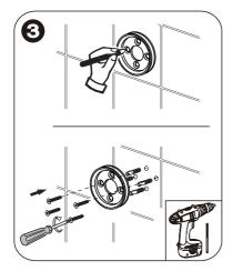
3. Using this mark as a guide mark 4 x fixing holes for the mounting bracket. Drill 4 x holes in the wall then insert the plastic wall plugs and attach the mounting bracket, using the supplied screws. Ensure the bracket is firmly attached to the wall.
