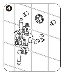
4. Place the chrome cover discs over the compression nuts on either of the shower mixer and align the mixer to the inlet pipes and onto the mounting bracket. (Make sure the red copper rings in compression nuts through the inlet pipes as well).
