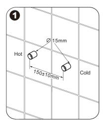
1.Leave 150±10mm between inlet pipework centers and about 25mm out from the finished wall surface.
