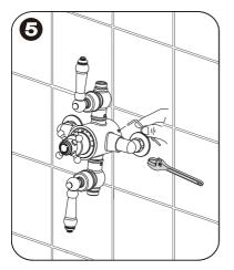
5. Carefully tighten up the compression nuts to hold the mixer in place. Ensure the shower mixer outlet is pointing in the correct direction (with the hot feed on the left side marked with a red indicator). Replace the locking grub screws to hold the mixer onto the wall bracket.
