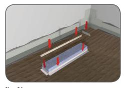
**Step 24**At this stage we recommend fitting tile trim to create a clean finished edge for the waste cover.
