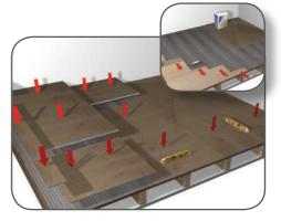
**Step 18**Repeat steps 17 and 18 for the remaining boards. Leave to set for approximately 3 to 5 hours.
