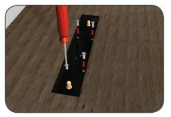
**Step 15**Line up the linear drain bowl with the drain top pre-fitted within the shower tray and connect the two together using the four bolts provided
