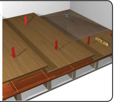
Measure, cut with a safety blade then lay Waterproof Matting in strips to cover the remainder of the floor area around the shower tray allowing a 50mm overlap over the Waterproof Matting strips and 50mm up the edges of each wall. Also allow a 50mm overlap over the shower tray edges. Set the strips of Waterproof Matting to one side.
