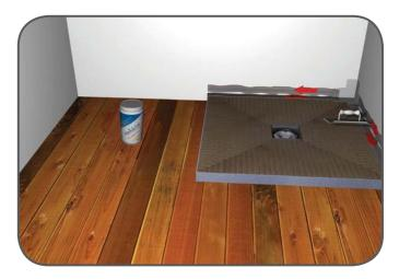
11. Where the shower area meets the wall apply a thin layer of Pro-SEAL tape sealer to the shower area and the adjoining wall approximately 60mm wide on both.
