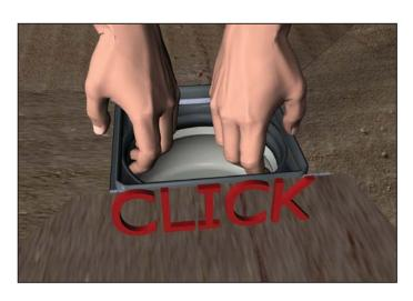
**Step 5**Put your fingers through the drain hole in the Shower Tray. Push down on the Shower Tray and pull the Shower Drain upwards until it clicks into place into the drain hole in the Shower Tray.
