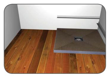
7. You will need to tape all joints where the tray meets an adjoining wall/s. Cut lengths from the roll of Waterproofing Tape and set aside for the moment.
