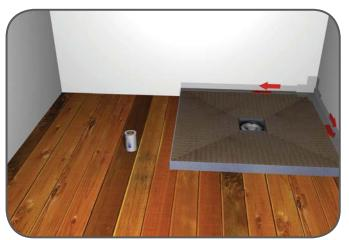
12. Place the strips of Waterproofing Tape previously cut in step 7 along the edges of the shower area, folding half up the wall and half on the shower area as you go. Press firmly into the Pro-SEAL tape sealer and the tape should also overlap the Waterproofing Internal Corners. When you have finished you can remove the protective gloves and eye and breathing protection.
