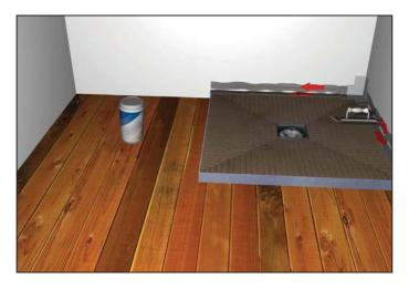
Step 11 Where the shower area meets the wall apply a thin layer of Pro-SEAL tape sealer to the shower area and the adjoining wall approximately 60mm wide on both.
