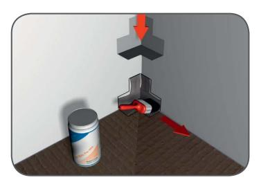
9. **Note:** Wear protective gloves, eye and breathing protection. Apply a thin layer of Pro-SEAL tape sealer to the internal corners of the shower area, slightly bigger than the pencil line marked in step 8.
