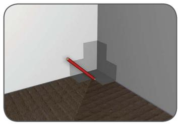
8. Temporarily place the Waterproofing Internal Corners into position and mark around them with a pencil. Once you have marked they can be set aside for the moment. This is to show where you need to apply the Pro-SEAL tape sealer.
