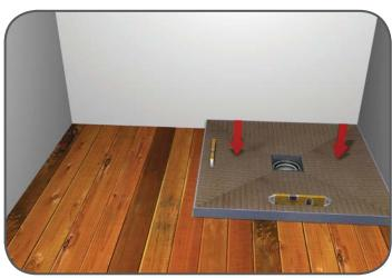
4. Place the Shower Tray into position and bed down onto the adhesive cement. Check that the shower tray is level in both directions using a suitable level.
