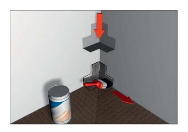
Note: Wear protective gloves, eye and breathing protection. Mix the 3.5kg Tub of Pro-SEAL tape sealer with 630ml of water in a clean bucket which will give the sealer a weak consistency. Using the
