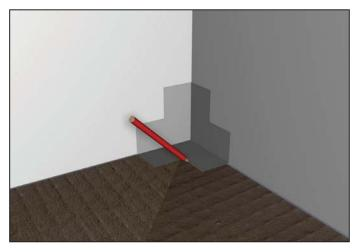
Step 8 Temporarily place the Waterproofing Internal Corners into position and mark around them with a pencil. Once you have marked they can be set aside for the moment. This is to show where you need to apply the Pro-SEAL tape sealer.
