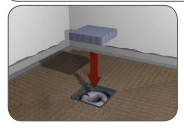
13. Place the Disposable Tiling Aid into the shower drain hole on the Shower Tray. The Tiling Aid provides the edge that needs to be tiled up to whilst protecting the Shower Drain from debris.
