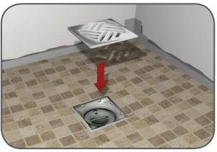
15. After tiling the Shower Tray, the Shower Drain Top can be fitted. Gently place the Shower Drain Top into the Shower Tray. Measure from the top of the finished tile to the top of the Shower Drain Top. From the opposite end/bottom of the Shower Drain Top mark the same distance as previously measured. Using a hard point saw, cut the excess from the bottom of the Shower Drain Top. Depending on your cutting skill, it may be necessary to file or sandpaper the cut edge to make it completely flat.
