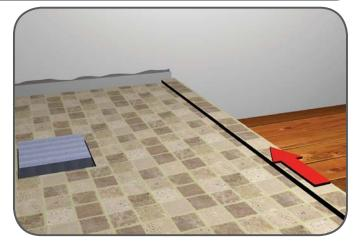
14. (Optional) After tiling the base of the shower area, we recommend that you add a further narrow border of tiles approximately 30mm to 40mm wide, along the top of the outside edge to act as a water retainer, stopping water running out of the shower area. The tiling aid can now be removed and disposed of.
