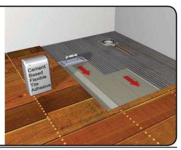
Apply an even thick wavy line of Fix MD Adhesive across all four edges of the shower tray. Place the shower tray into position and bed down onto the adhesive. Check that the shower tray is level in both directions along the edge using a suitable level.
