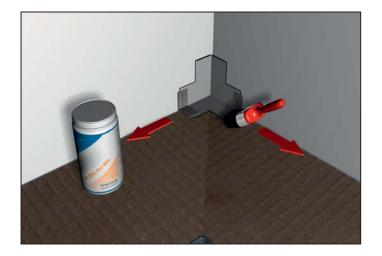
Step 10 Place the Waterproofing Internal Corners into the internal corners of the shower area and push firmly into the Pro-SEAL tape sealer. Apply a further thin layer of Pro-Dry tape sealer over the edges of the waterproofing internal corners.
