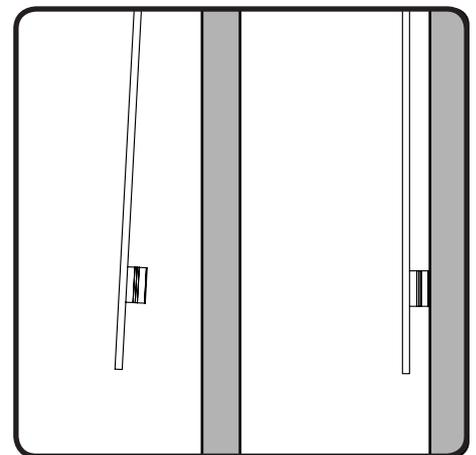
8. The wall spacer can be screwed to the wall if the mounting surface is unsuitable for fixing with adhesive tape.
