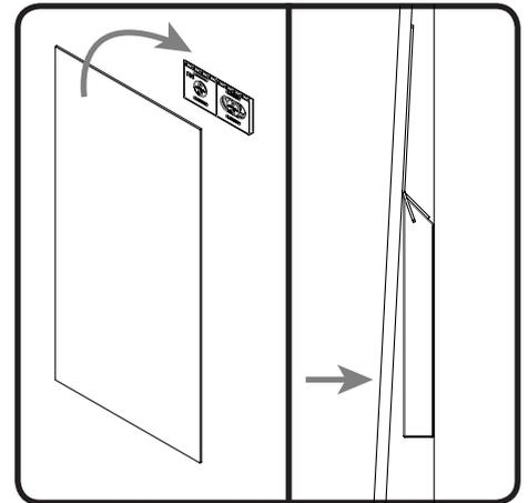
6. Peel the protective cover strip from the double sided tape on the support brackets.
