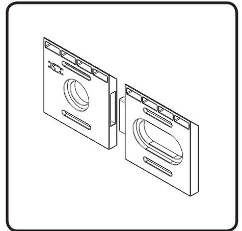
2. Place the bottom edge of the Hang 'N' Lock bracket onto the reference line and mark a screw hole position in each cam hole recess. Remove the bracket from the wall.
