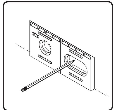
3. Drill holes to a depth of 45mm and insert the wall plugs level with the surface of the wall. (Note: if you are fitting the product to a tiled surface, insert the wall plugs below the surface of the tile to avoid cracking the tiles). Insert the countersink screws through the Hang 'N' Lock cams and loosely secure the Hang 'N' Lock bracket to the wall.
