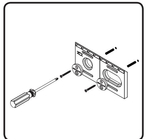
4. With the Hang 'N' Lock bracket loosely attached to the wall, adjust for height and level by rotating the cams with a flat head screwdriver, then use a Philips screwdriver to fully tighten the mounting screws, to securely fix the bracket into position.
