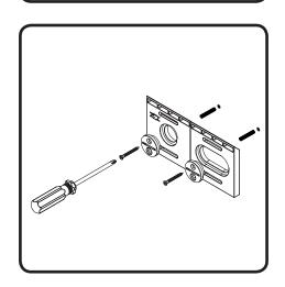
4. With the Hang 'N' Lock bracket loosely attached to the wall, adjust for height and level by rotating the cams with a flat head screwdriver, then use a Philips screwdriver to fully tighten the mounting screws, to securely fix the bracket into position.
