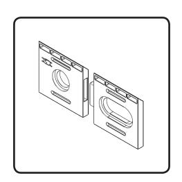
2. Place the bottom edge of the Hang 'N' Lock bracket onto the reference line and mark a screw hole position in each cam hole recess. Remove the bracket from the wall.
