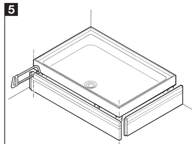
If necessary, carefully cut the outside edges of the panel/s to fit.
