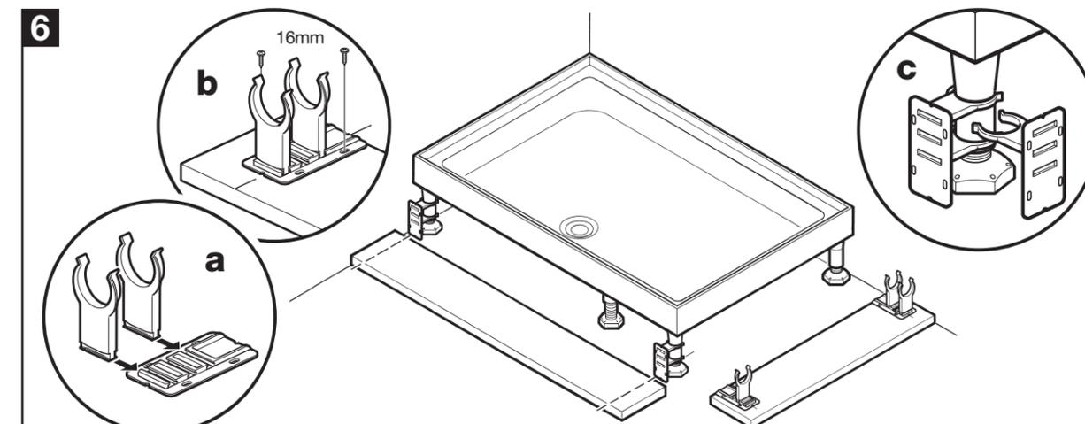
(a) Separate and assemble the panel brackets. Push fit the panel brackets onto the legs, align panel/s up with the brackets and mark the centre line of the brackets onto the back of the panel/s.
