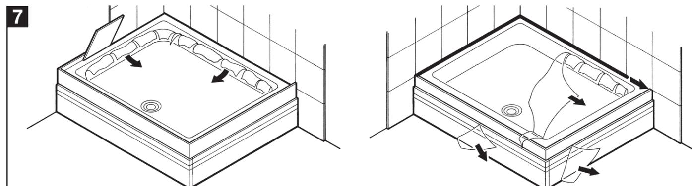
Peel back protective film from back edges of tray. **Tile over the upstands. Seal the wall edges of tray with silicone sealant.** When the final installation of the enclosure is complete, remove the remaining protective film.
