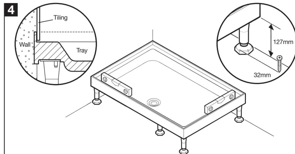
Ensure the tiling upstands are either recessed into the wall or boarded over so the tiling face is flush with the edge shown in the diagram. Adjust legs where necessary. Check tray is level in all directions (there is a built in fall on the tray for water drainage). Ensure all legs are wound down tight to the floor. Fix legs to the floor using 32mm screws, where accessible.
