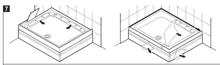
Peel back protective film from back edges of tray. **Tile over the upstands. Seal the wall edges of tray with silicone sealant.**When the final installation of the enclosure is complete, remove the remaining protective film.
