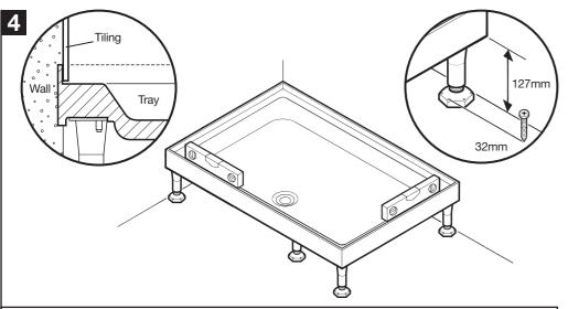
Ensure the tiling upstands are either recessed into the wall or boarded over so the tiling face is flush with the edge shown in the diagram. Adjust legs where necessary. Check tray is level in all directions (there is a built in fall on the tray for water drainage). Ensure all legs are wound down tight to the floor. Fix legs to the floor using 32mm screws, where accessible.
