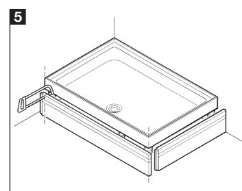
If necessary, carefully cut the outside edges of the panel/s to fit.
