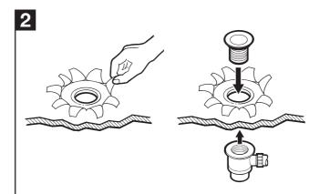
Peel back protective film from waste hole inside the tray and fit waste outlet. Fit the waste and trap as per the manufacturers instruction. **Do not apply any sealant to the underside of the tray as this will invalidate the guarantee.**
