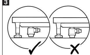
Place the tray in position and fit waste pipe. Make sure pipe work is clear of floor when standing in the tray. If necessary cut a hole in the floor to provide adequate clearance.
