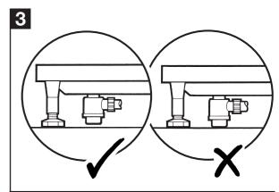
Place the tray in position and fit waste pipe. Make sure pipe work is clear of floor when standing in the tray. If necessary cut a hole in the floor to provide adequate clearance.
