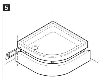
If necessary, carefully cut the outside edges of the panel to fit.
