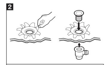
Peel back protective film from waste hole inside the tray and fit waste outlet. Fit the waste and trap as per the manufacturers instruction. Do not apply any sealant to the underside of the tray as this will invalidate the guarantee.
