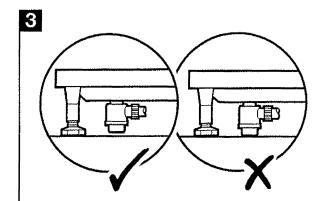
Place the tray in position and fit waste pipe. Make sure pipe work is clear of floor when standing in the tray. If necessary cut a hole in the floor to provide adequate
