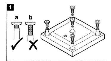
Fit ALL legs, including the centre leg. NOTE: The legs must be screwed in far enough that the end of the groove on the leg is NOT visible (a).
