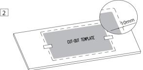
Drill holes inside the cutting line to allow access for a saw.
