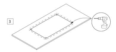
Drill holes inside the cutting line to allow access for a saw.
