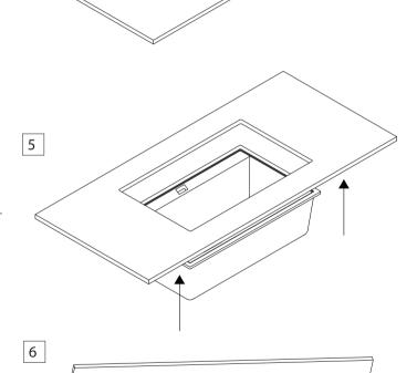
Bring the sink up to the cutout and mark the positions to place the allotted clips. Use the clips as a guide to mark the drilling positions.
