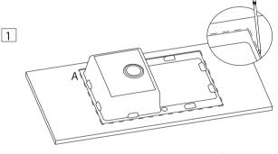
Using a pencil, draw around the sink accurately. Remove the sink and draw another line 10mm inside the sink top outline. This is the cutting line for the opening. If a template is supplied simply draw around the edge of the template.
