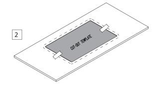
Place the cut-out template centrally inside the marked perimeter and mark the cut-out perimeter with a pencil.This will be your cut-out guide.
