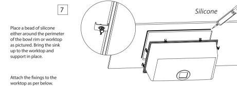
**Clip Fixing** affix all clips to clip mounting positions. Do not overtighten screws – tighten by hand.
