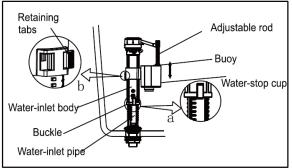
Put fill valve and water inlet triangle washer inset into water inlet hole of water tank, then, cover water inlet flat waste, plastic washer and hexagonal nut in turn from the bottom of the fill valve. Fastening water inlet hexagonal nut and make a proper adjust according to the size of water tank.
