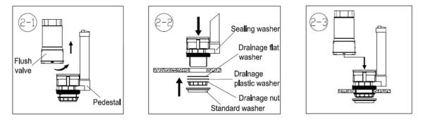
2-1 Circumrotate drainage body and remove it from the pedestal.
