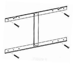
Hang the appliance onto the hooks at the bottom of the bracket and push the top of the appliance into the mounting bracket. Now fix the appliance to the mounting bracket by refitting the two screws which were removed at the beginning.
