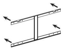
Take away the mounting bracket and then drill four 8mm diameter holes on the wall. Insert the plastic wall plugs into the drilled holes. If installing the appliance on a solid wood wall there is no need to drill the holes in the wood and no need for the plastic wall plug. Fix the mounting bracket using the four screws provided.
