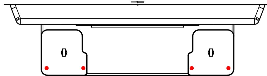
Straighten up the adjustment covers and screw in **ONE** Screw per adjuster while holding the seat in the correct position.
