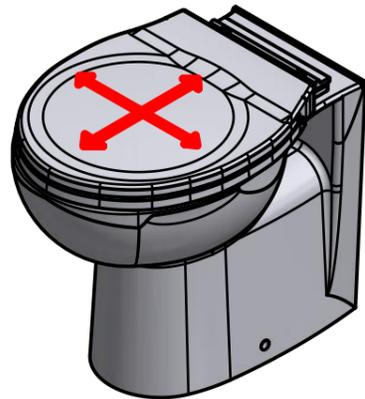
While the lid is clamped down, slide it to your preferred position on the toilet pan. Hold the base of the hinge while opening the handle to reveal the adjuster plates.
