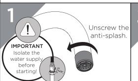
Remove the anti-splash and filter from housing. Clean and replace as necessary.
