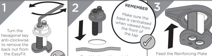
Feed the base through the sink hole from the top.
