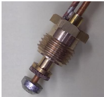
Connection to gas valve
