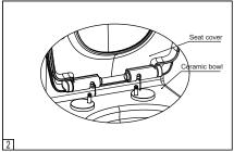
2.Attach the seat cover into hinge bar as per drawing.
