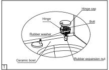
1.Insert rubber expansion nut into bowl bolt holes then install hinge and bolt into hinge holes. Using screwdriver to tighten the bolt into rubber expansion nuts and close the caphinge.
