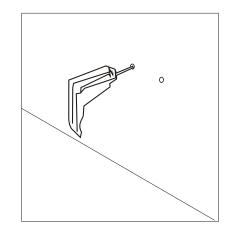
2) Someone holds the bsain on its place ,the other one remove the pedestal away,then put marks on the wall for the installing holes (two).
