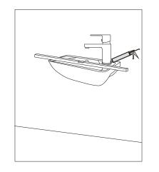
3) Take away the basin, use Ø10mmdriller to make two 60mm depthholes following the marks.
