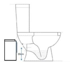
This macerator is only for use with a toilet using a horizontal outlet. The toilet must also have a flushing tank or tap. Note: the horizontal outlet must be 18cm above floor level in accordance with EU standards.
