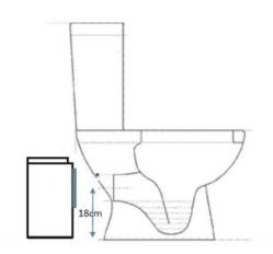
This macerator is only for use with a toilet using a horizontal outlet. The toilet must also have a flushing tank or tap. Note: the horizontal outlet must be 18cm above floor level in accordance with EU standards. <u>Customer Care Helpline</u> Telephone: 01386 800750 Email: <u>technical@plumbworld.co.uk</u>
