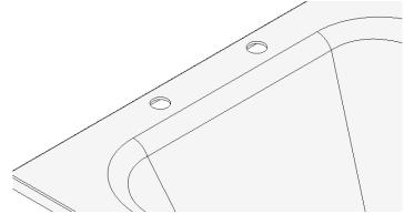
Drill the holes 180mm apart with a 28-30mm hole saw.
