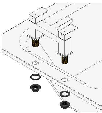
Place the washer on the tap barrel, then tighten the tap to the bath with the back nuts.
