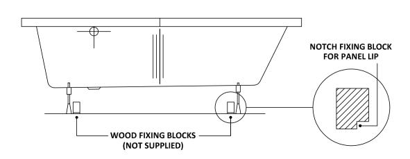
4. MARK DIMENSION 'A' LIGHTLY WITH A PENCIL AND USING A FINE TOOTHED SAW, CAREFULLY TRIM THE END PANEL TO LENGTH. IT IS RECOMMENDED THAT A WALL BATON IS FITTED BEHIND THE CUT END FOR SUPPORT AND A WOODEN BATON FLOOR MOUNTED TO PREVENT THE PANEL FROM MOVING INWARDS.
