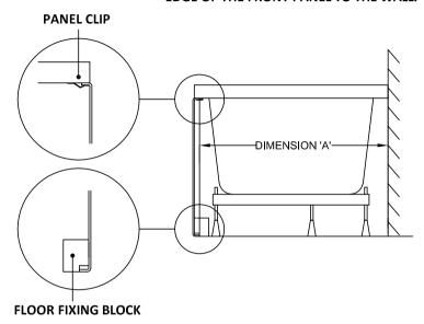
2. MEASURE THE HEIGHT OF THE PANEL, AND SET THE BATH TO THIS DIMENSION FROM THE FLOOR TO THE UNDERSIDE OF THE BATH RIM.
