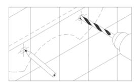
1. Use pencil to mark desired fixing location, using the holes in the washbasin as a guide. Check wall plug dimension and use corresponding bit size to drill as required, ensure the basin is true using the spirit level before drilling.
