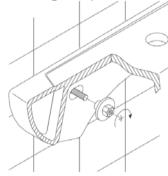
3. Offer basin up to bolts, fit nylon spacer and tighten nut. Please Note: On some fixings the nut maybe incorporated into the spacer.
