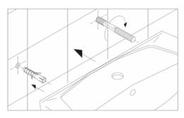
2. Insert plugs in to both holes. Fix bolts into plugs.
