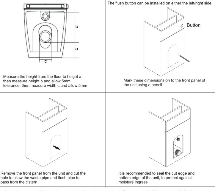
Note: For safety reasons Unit must be secured to the wall using suitable fixings (pre-drilled holes provide in back panel of unit)Please note-wall fixings are not supplied These can be purchased from a local DIY store
