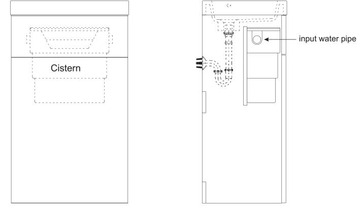
input water pipe can be Right/Left option as valve position
